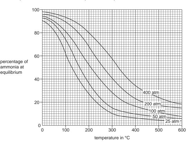
The reaction requires the use of a catalyst, which operates most efficiently within the temperature range 280 - 450 °C.
